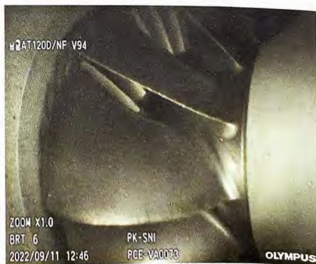
Photo of First Stage Compressor 2 nd Quadrant
