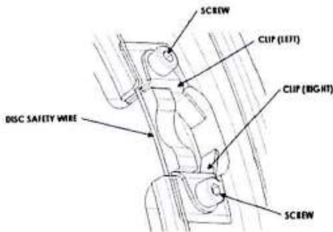
**CAUTION:** Disc safety wire must be in place, it prevents disc from sliding out the slots.
