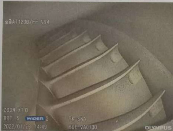
Photo of Leading Edge CT-Blades 3 rd Quadrant
