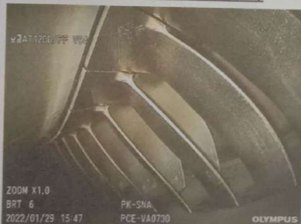
Photo of CT-Blades Trailing Edge3 rd Q
