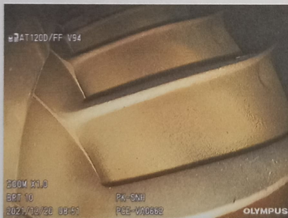
Photo of Leading Edge CT-Blades 3 rd Quadrant
