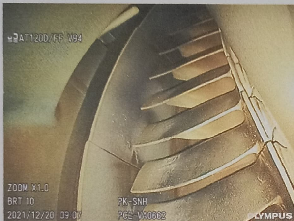
Photo of CT-Blades Trailing Edge 1 st
