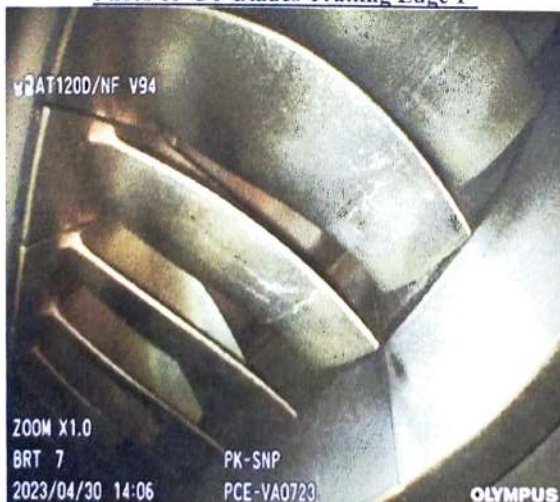
Photo of CT-Blades Trailing Edge 1 st
