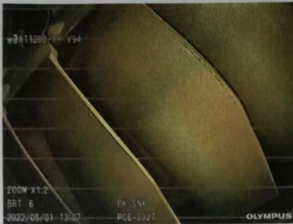
Photo of CT-Blades Trailing Edge 3 rd Q
