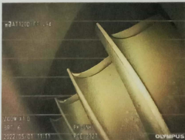
Photo of Leading Edge CT-Blades 1 st Quadrant
