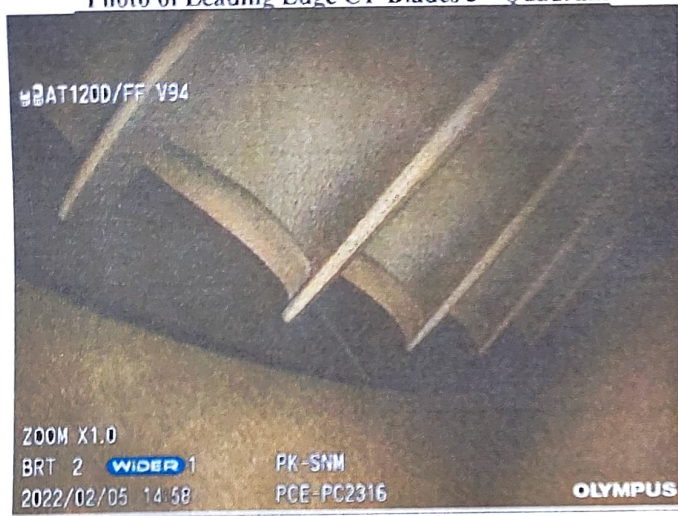
Photo of Leading Edge CT-Blades 3 rd Quadrant
