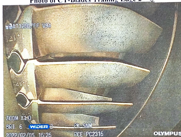
Photo of CT-Blades Trailing Edge 2 nd Q
