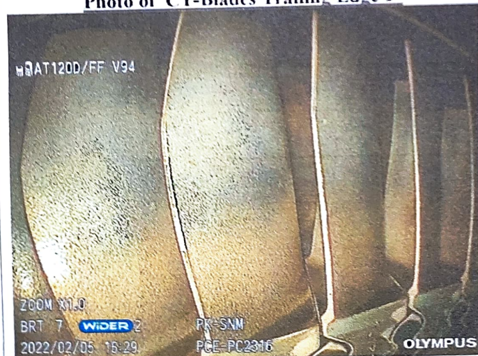
Photo of CT-Blades Trailing Edge 1 st
