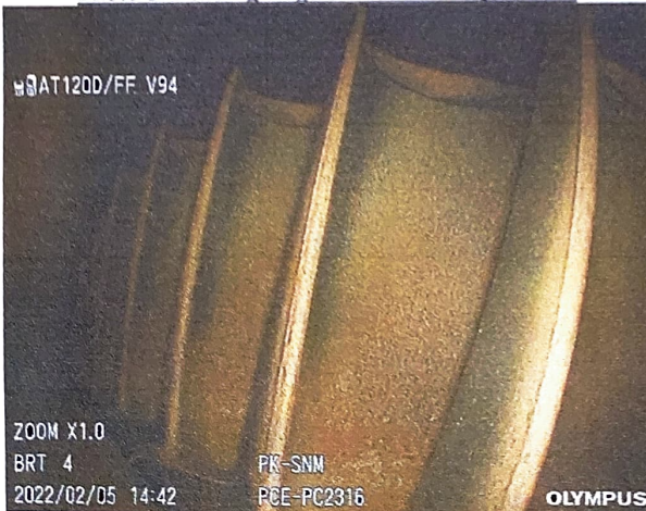
Photo of Leading Edge CT-Blades 1 st Quadrant
