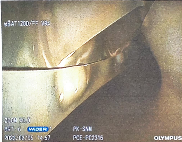
Photo of CT Stator 3 rd Quadrant
