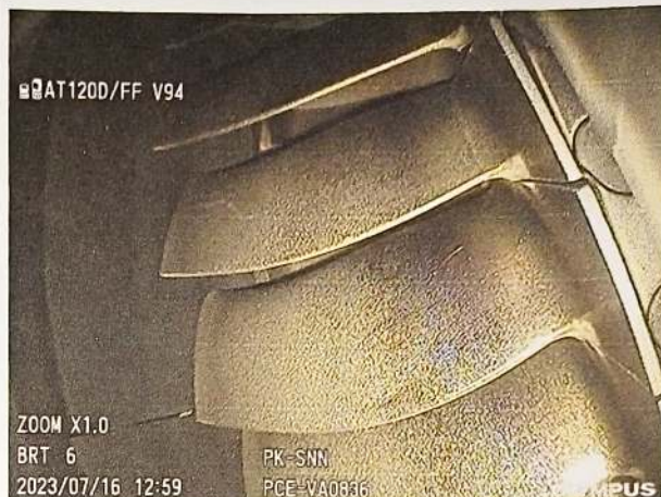
Photo of CT-Blades Trailing Edge 4 th Q
