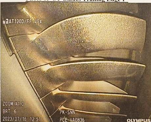
Photo of CT-Blades Trailing Edge 1 st
