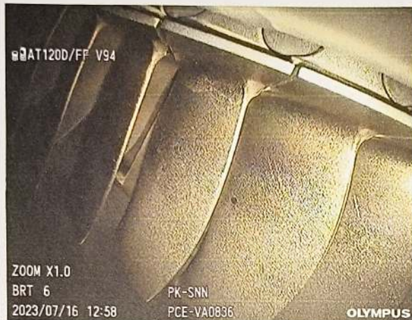
Photo of CT-Blades Trailing Edge 3 rd Q
