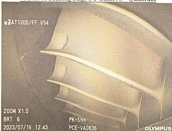
Photo of Leading Edge CT-Blades 3 rd Quadrant
