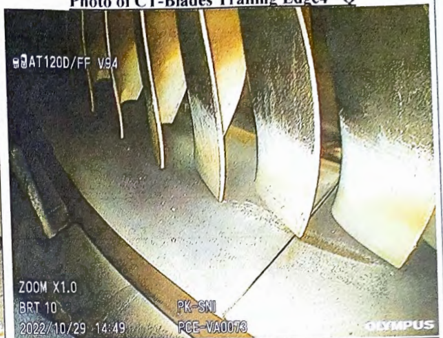
Photo of CT-Blades Trailing Edge 4 th Q
