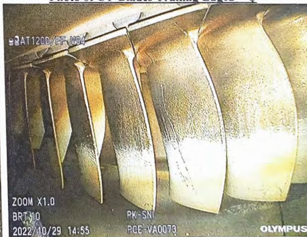
Photo of CT-Blades Trailing Edge 2 nd Q
