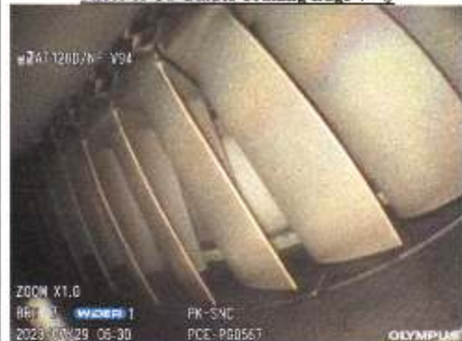
Photo of CT-Blades Trailing Edge 4 th Q
