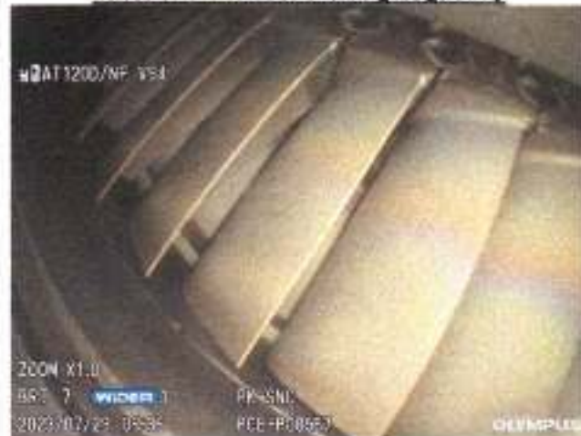
Photo of CT-Blades Trailing Edge 3 rd Q
