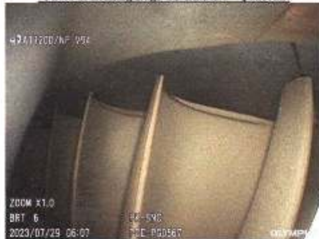
Photo of Leading Edge CT-Blades 3 rd Quadrant
