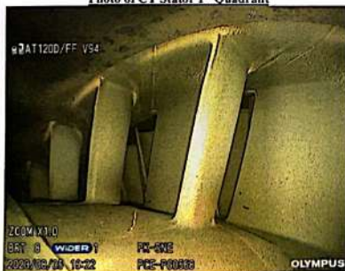
Photo of CT Stator 1 st Quadrant
