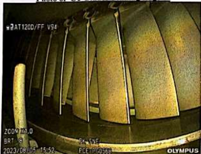
Photo of CT-Blades Trailing Edge 1 st
