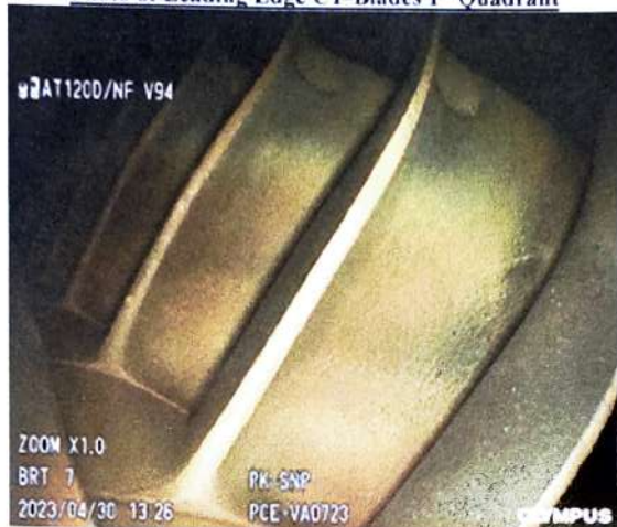
Photo of Leading Edge CT-Blades 3 rd Quadrant
