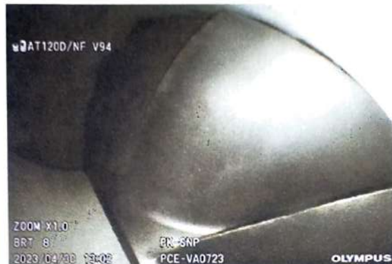
Photo of First Stage Compressor 3 rd Quadrant
