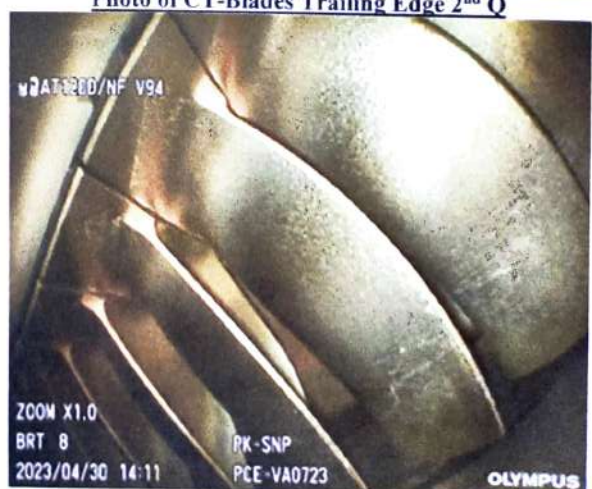
Photo of CT-Blades Trailing Edge 2 nd Q
