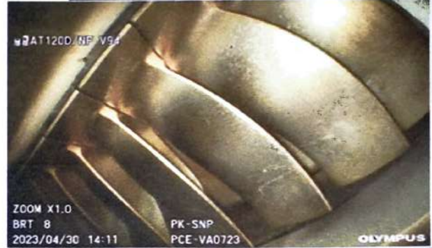
Photo of CT-Blades Trailing Edge 4 th Q
