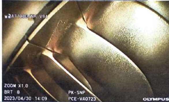
Photo of CT-Blades Trailing Edge 3 rd Q
