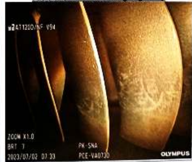
Photo of CT-Blades Trailing Edge 2 nd Q
