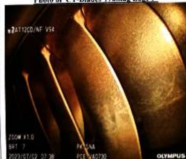
Photo of CT-Blades Trailing Edge 1 st
