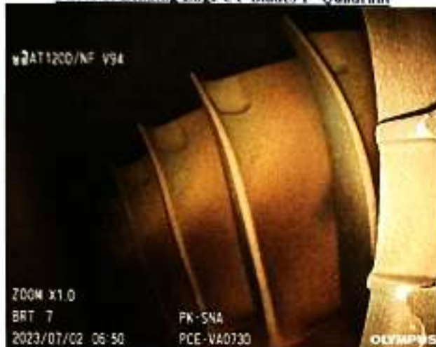
Photo of Leading Edge CT-Blades 3 rd Quadrant
