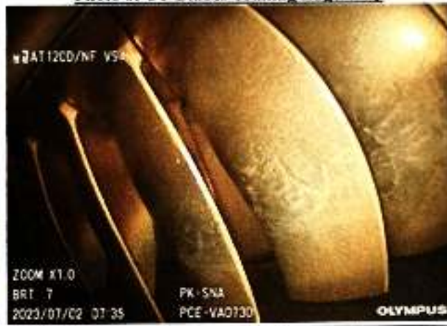
Photo of CT-Blades Trailing Edge 4 th Q
