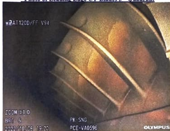
Photo of Leading Edge CT-Blades 3 rd Quadrant
