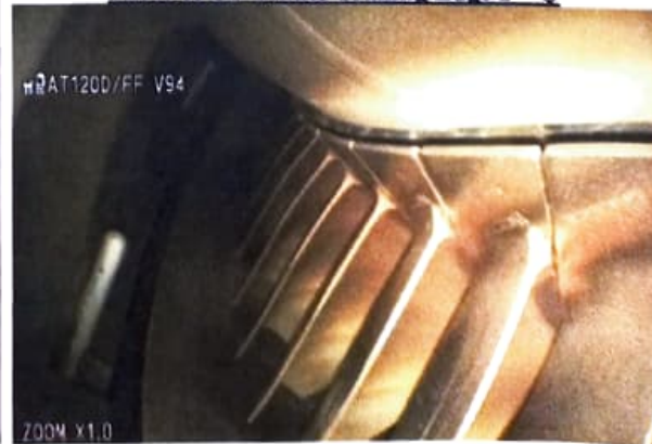
Photo of CT-Blades Trailing Edge 2 nd Q
