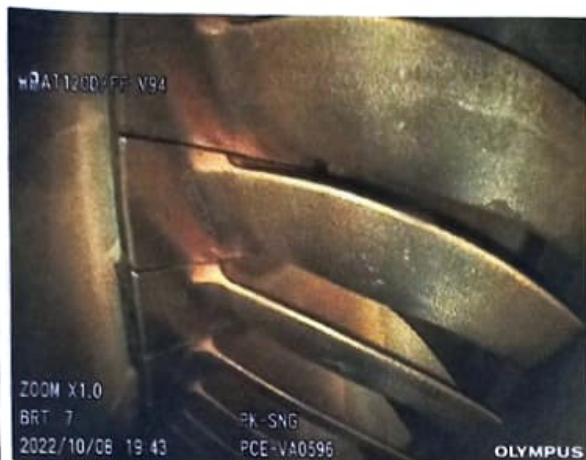
Photo of CT-Blades Trailing Edge 3 rd Q
