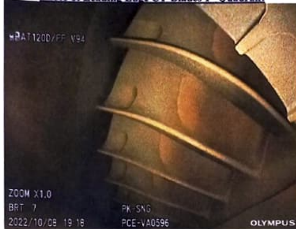
Photo of Leading Edge CT-Blades 3 rd Quadrant
