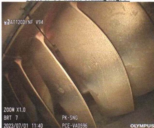
Photo of CT-Blades Trailing Edge 1 st
