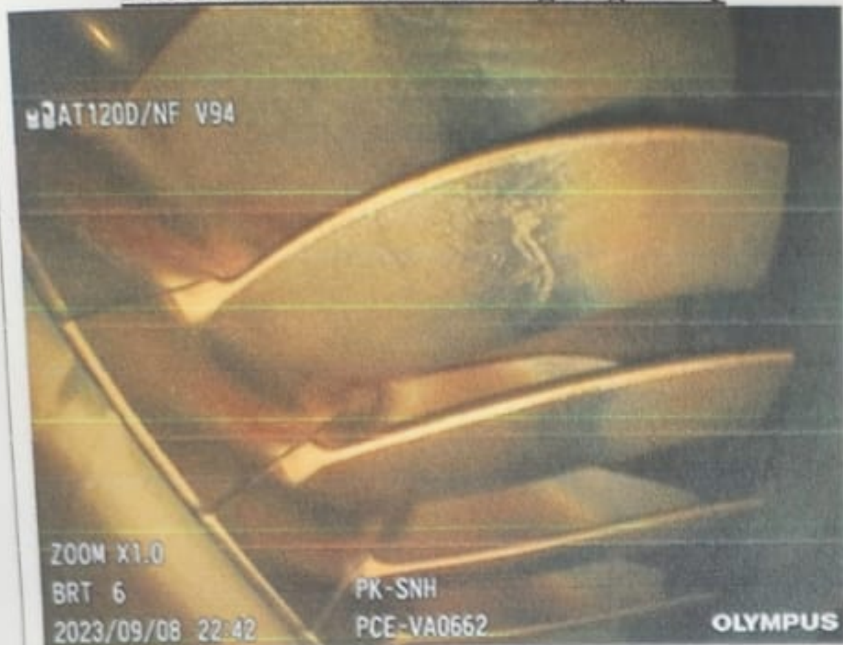
Photo of CT-Blades Trailing Edge 3 rd Q
