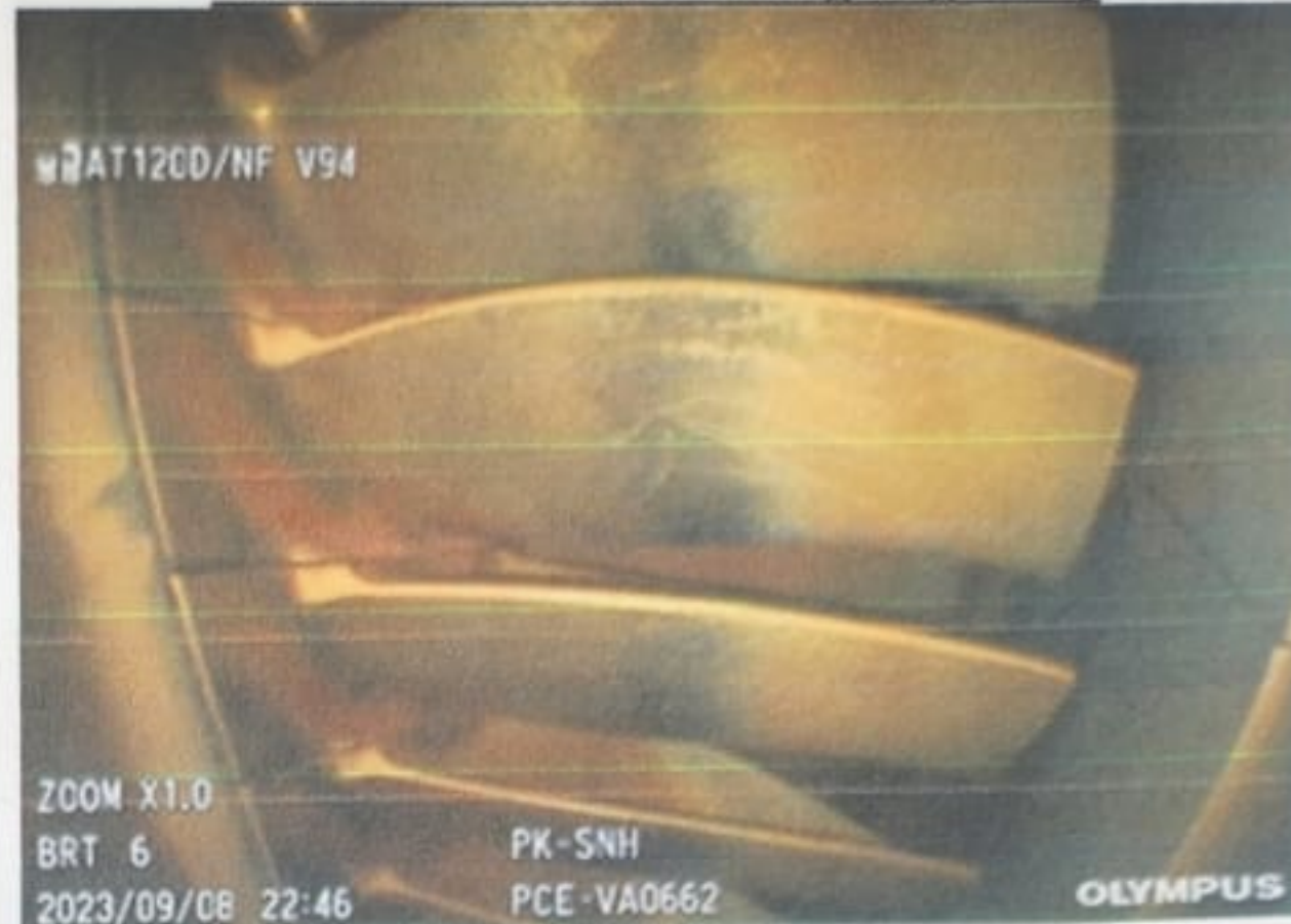
Photo of CT-Blades Trailing Edge 4 th Q
