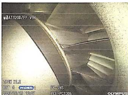
Photo of First Stage Compressor 4 th Quadrant
