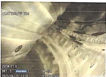
Photo of Combustion Chamber 4 th Quadrant
