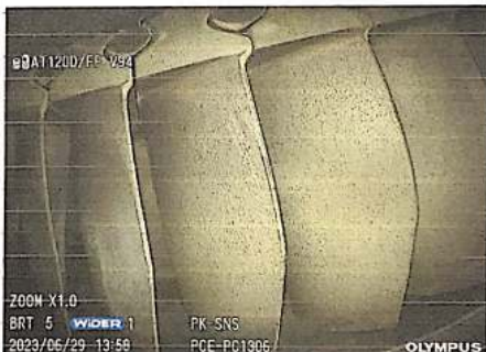
Photo of CT-Blades Trailing Edge 4 th Q
