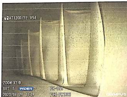
Photo of Leading Edge CT-Blades 1 st Quadrant
