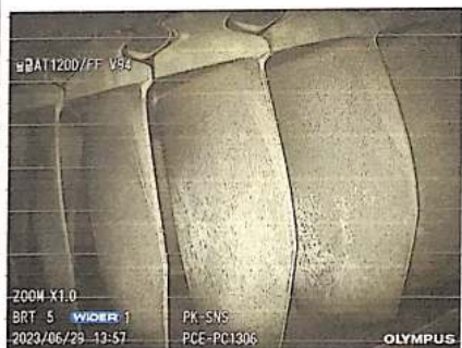
Photo of CT-Blades Trailing Edge 1 st
