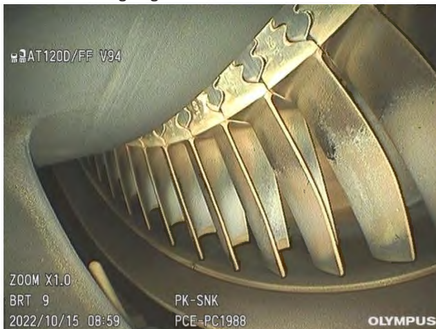
Photo of Trailing Edge CT-Blades 1 st Q
