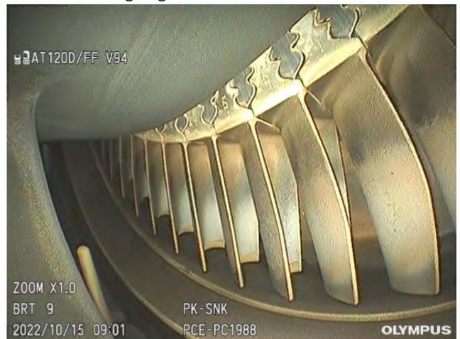
Photo of Trailing Edge CT-Blades 2 nd Q
